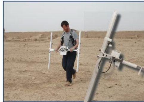
Grad601 Single axis fluxgate gradiometers For detection of shallowly buried material - Easy electronic adjustment of the sensors
