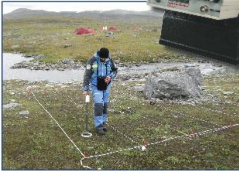
MS2 Magnetic susceptibility measurements For field and laboratory applications - Susceptibility to 2 \times 10^{-6} SI resolution
